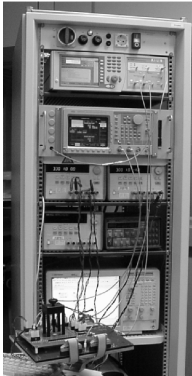
Figure 5.11: Photograph of the test setup for characterizing the A/D converters designed in this book
