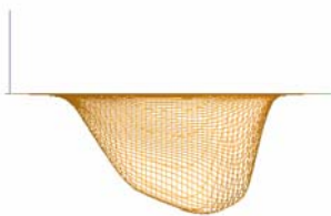
Fig. 1: Scan strategy and final shape of the surface after milling a hole with pixels confined to a circle. The surface is shown in 3D view and in its projection to the x-z and y-z plane. (a) raster scan, single pass, (b) spiral scan, single pass, (c) spiral scan, multi pass.
