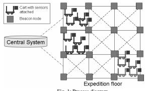
Fig. 1: Process diagram. Carts gather on allocated grid rectangles within the expedition floor.
