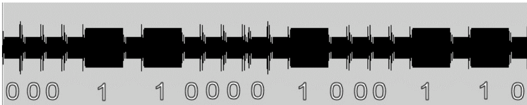
Figure 4: An SPA attack on a power trace of a straightforward RSA implementation.
