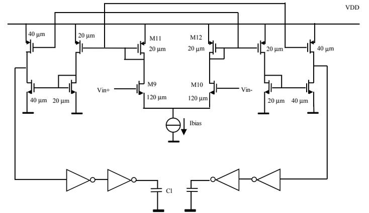
Figure 4 Differential driver stage.
