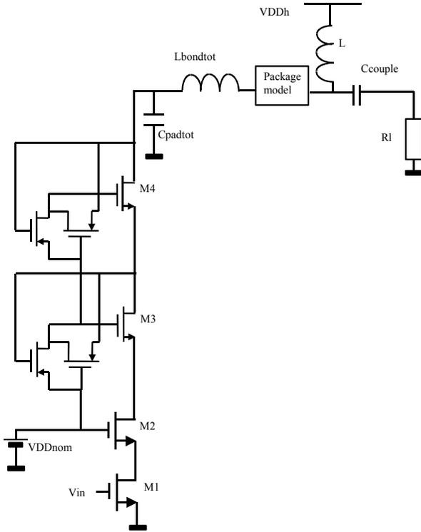
Figure 3 Single ended PA output stage.
