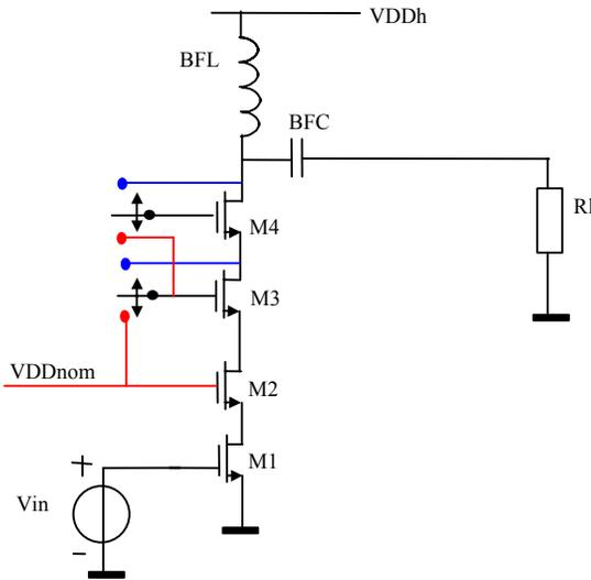
Figure 1 Switched cascode implementation in a PA.
