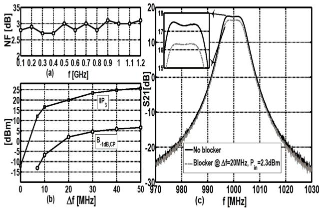
Fig.5: a) NF of the filter at different clock frequency; b) IIP<sub>3</sub> and  $B_{1dB,CP}$  for different offset frequencies; c) Transfer function of the filter at  $f_{lo}$ =1GHz with and without CW blocker with  $P_{in}$ =2.3dBm located at  $\Delta f$ =20MHz from center frequency
