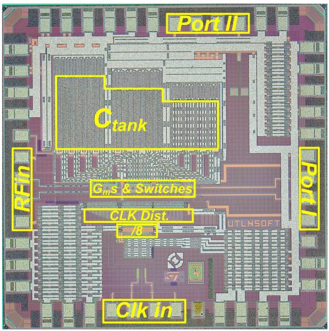
Fig.7: Chip micrograph
