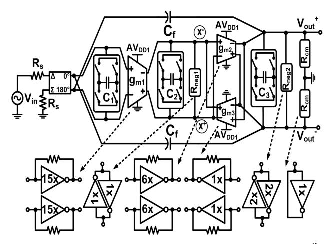
Fig.2: Schematic of a proposed widely tunable  $6^{th}$  order  $g_m$ -switched-C BPF
