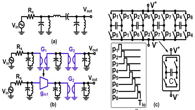
Fig.1: a) A conventional singly terminated 6<sup>th</sup> order LC BPF b) Exploitation of gyrators to transform a series LC tank to parallel one c) each LC tank is emulated by a differential switched-capacitor 8-path filter
