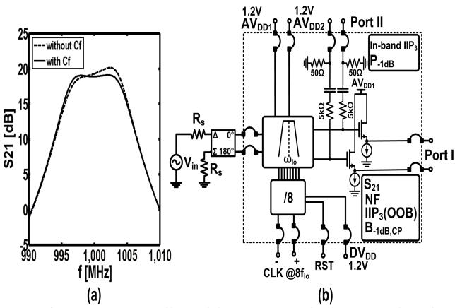
Fig.3: a) The simulated effect of C<sub>f</sub> on the transfer function of the filter b) Measurement interface
