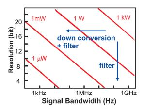
Figure 2: Power consumptions of ADC's as a function of signal bandwidth and resolution
