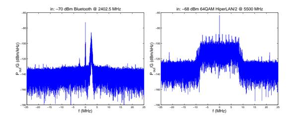
Figure 5: Measured output spectra of the receiver. Left: Bluetooth. Right: HiperLAN/2.
