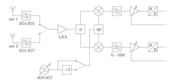
Figure 4: A Software Defined Radio with switchable RF filters
