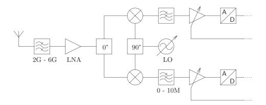
Figure 3: A Software Defined Radio with one wide RF filter
