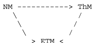
Figure 1: PCN Codepoint Re-Marking Diagram for Dual Marking (DM)
