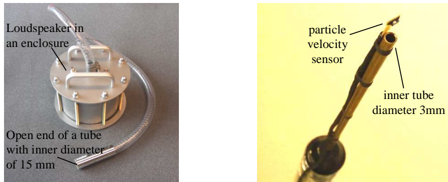
Figure 2. Left: Mid-high frequency monopole. Right: extension piece and miniature reference sensor.
