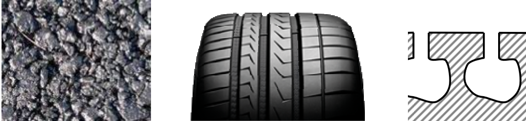
Figure 1. Holes in the pavement (left) and groves in the tyre (middle) form cavity resonators (right).
