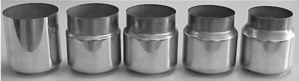
Figure 3. Products used for the tests made by deep drawing, wall ironing and necking; the diameter is 66 mm. Tensile test specimens were cut from the upper, necked part in tangential direction.
