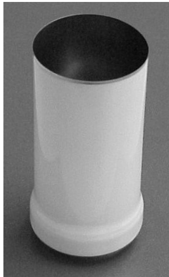
Figure 1. A two-piece can in early production stage, the diameter has been reduced from 66 mm to 62 mm over a large part of the height (body-necked).
