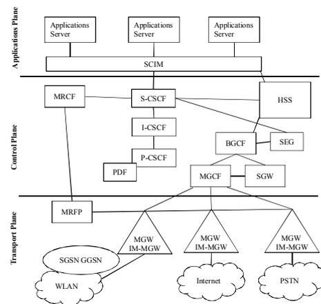
Figure 3 Simplified IMS reference architecture [9]
