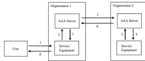
Figure 5 End-to-end AAA solution
