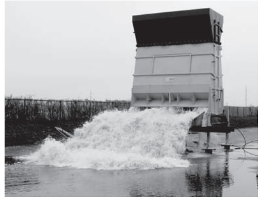
Figure 2. Enlarged overtopping simulator (22 m 3 ).
