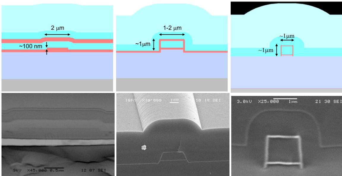
**Fig. 3:** Schematics (top) and corresponding SEM pictures of realized structures (bottom) of three typical channel layouts: a non-symmetrical layout with very large modal birefringence (left), an A-shaped layout with strongly reduced modal birefringence (center) and a box-shaped layout with minimal modal birefringence (right). The nitride layers are shown in red in the schematic view.
