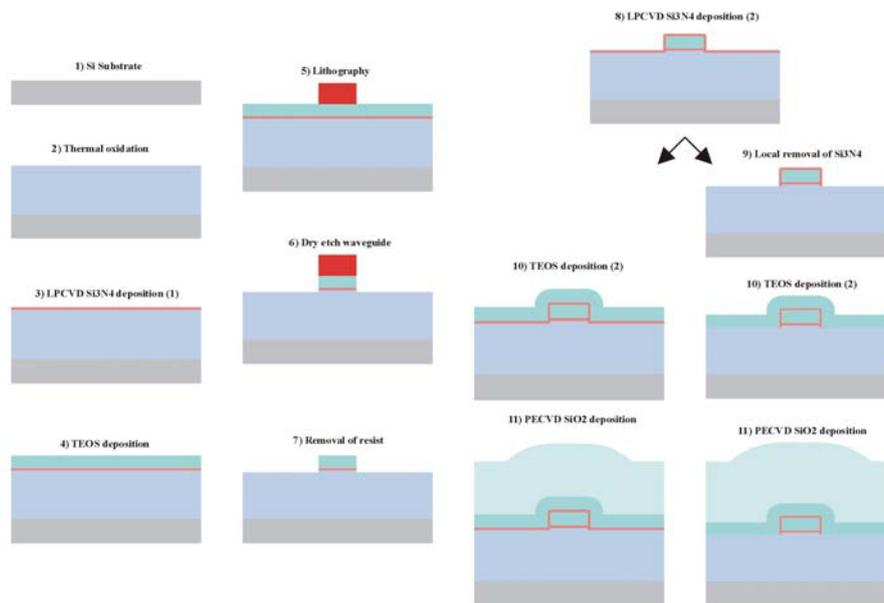
**Fig. 2:** Flow process scheme as made with Flowdesigner process modeler (PhoeniX BV, Enschede, the Netherlands). Here, the  $\text{Si}_3\text{N}_4$  is shown in red, and the (different types of)  $\text{SiO}_2$  in blue. For explanation, see text.
