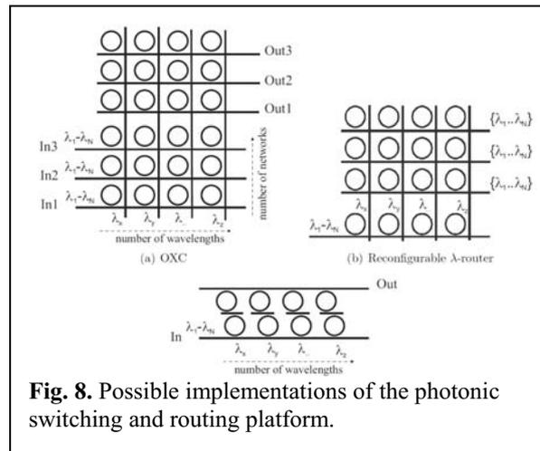
Fig. 8. Possible implementations of the photonic switching and routing platform.
