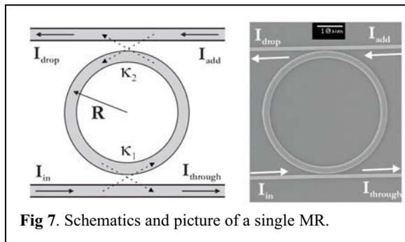
Fig 7. Schematics and picture of a single MR.
