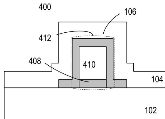
**Fig. 1:** Cross-section of a typical waveguide structure, with LPCVD  $\text{Si}_3\text{N}_4$  (in grey) as basic waveguiding layer, filled with and in turn encapsulated by  $\text{SiO}_2$  (white). Figure extracted from [7]
