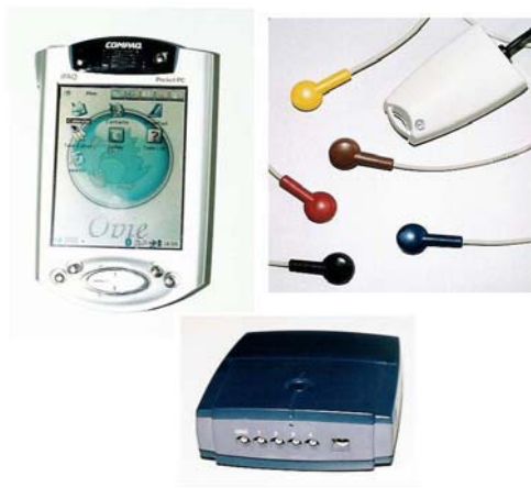
Fig. 3b. One BAN configuration: PDA, front-end and sensors
