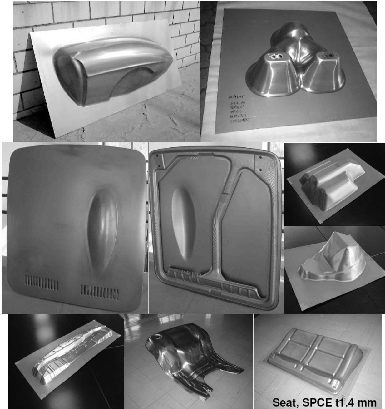
Figure 14. A collection of parts (mostly automotive) made by Incremental Sheet Forming (courtesy Amino North America Corporation, www.aminonac.ca ).
