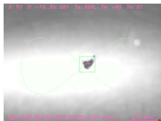
Figure 4: Screenshot of the particle tracking program where the green square indicates the particles that is manipulated and the pink lines represent the x- and y-position vectors given by the controller output.
