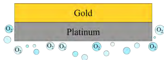
Figure 8: Schematic view of the gold wire coated by platinum where only bubbles are formed on the platinum surface
