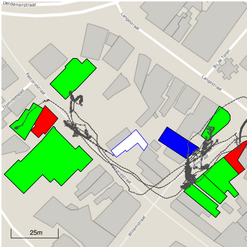
Figure 1: Trajectory annotation using Point-of-Interest Extraction (PIE). Green, blue and red polygons indicate the footprint of POIs that were extracted as visited. White and grey polygons were not extracted as visited. For green polygons proof was available of a visit, blue and white polygons were possibly visited, and red and grey polygons were definitely not visited in the real world.
