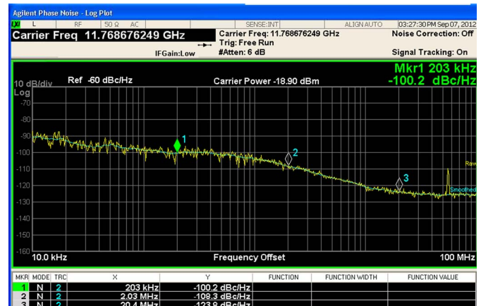
Fig. 5. Measured phase noise at 11.8GHz carrier frequency
