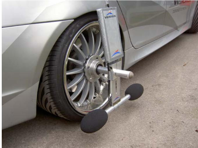
Figure 1 – CPX measurement set-up.
