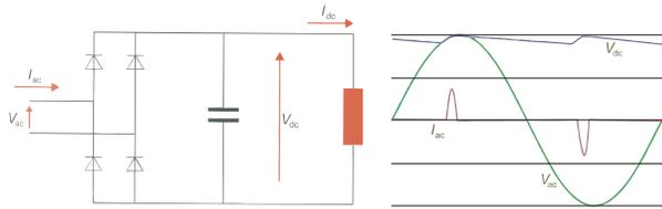
Fig. 2. Conventional rectifier (left) and its terminal voltages and currents (right) [14]
