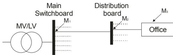
Fig. 8. Schematic of distribution of power supply in Carré: M<sub>1</sub>, M<sub>2</sub> and M<sub>3</sub> designate the measurement locations
