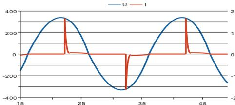
Fig. 3. Current consumption (red) of dimmer
