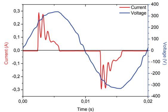
Fig. 4. Measured waveforms 11W CF light
