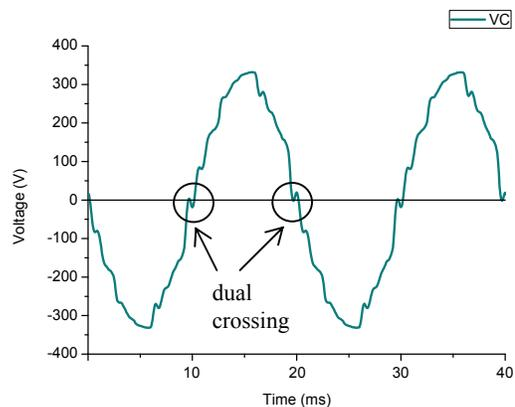
Fig. 6. Measured distorted voltage waveform
