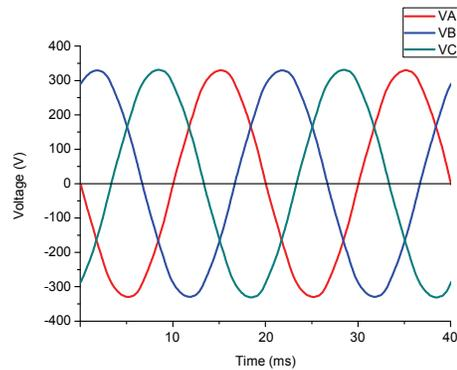
Fig. 10. Measured voltage waveforms transformer without load
