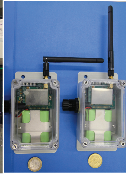
Fig. 4. Two CC2430 radio's
