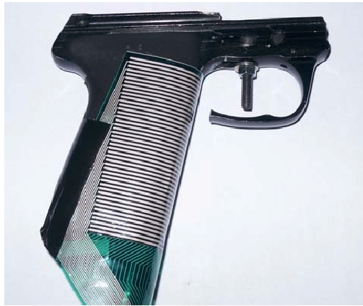
Fig. 3. The sensor wrapped around the gun's butt.
