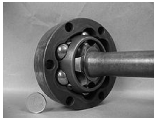
Figure 3. Rzeppa constant velocity joint.
