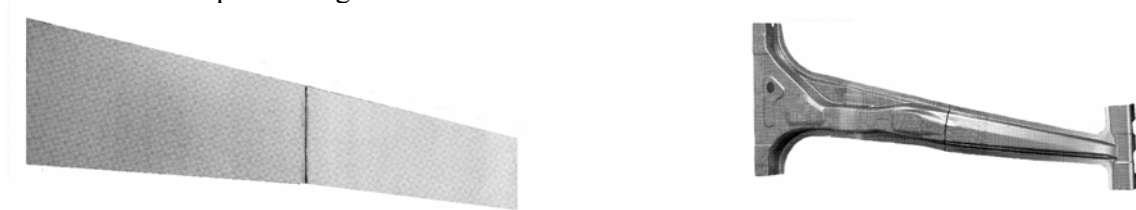
Figure 1. Tailored Blank for B-pillar
