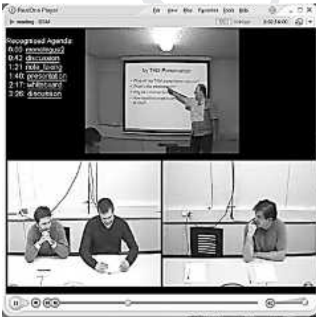
Fig. 9.3 The three camera views of the M4 meeting corpus, and a sequence of automatically recognized speaking turn patterns (top left) with the HMM approach proposed (McCowan et al. , 2005b).
