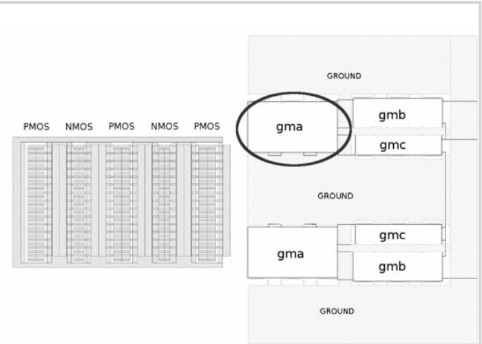
Figure 21.3.2: Partial layout floor plan of a single inverter (left) and transconductor (right).
