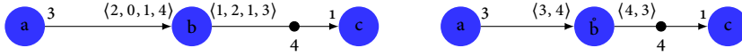
FIGURE 6.6 – Applying the vectorisation transformation to an actor groups together several consecutive firings into a single firing, by replacing the rates of these firings with their sums. In the graph above, actor b is vectorised by applying a blocking vector of (3, 1) .
