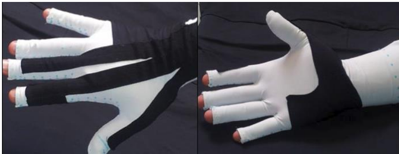
Figure 14. Glove design. KPF goniometers were integrated in the metacarpal-phalangeal area of thumb, index and medium fingers. Force sensitive resistors were integrated in the palm, lateral side of the glove and the lateral side of the middle phalanx of the forefinger.
