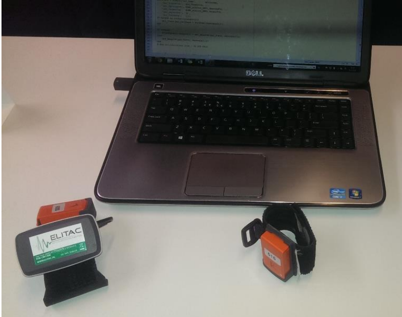
Figure 34. AUC prototype. In the picture, two Xsens MTw (orange boxes) and one Elitac module are shown.
