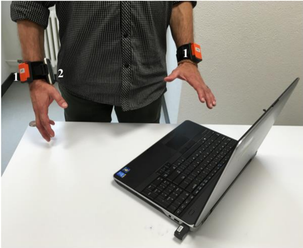
Figure 37. Right impaired stroke subject with AUC prototype. 1. Inertial sensors; 2. Elitac VT actuator.
