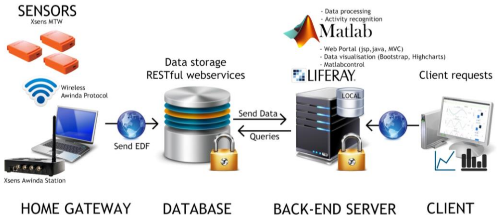
Figure 10. System Architecture. The home gateway captures sensor data and sends it in an EDF to a secure database. Portal technology can access and process the data and visualize the results to care-professionals on a web-portal.
