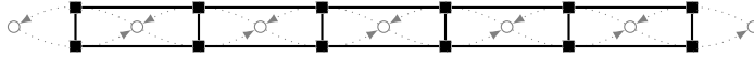
(a) Constraint graph (E, \mathcal{J}_{B/M}) for the line network, where E is represented by square shaped nodes and \mathcal{J}_{B/M} by solid lines. Moreover, the line network (V, E) is depicted by circle shaped nodes and dotted lines.
