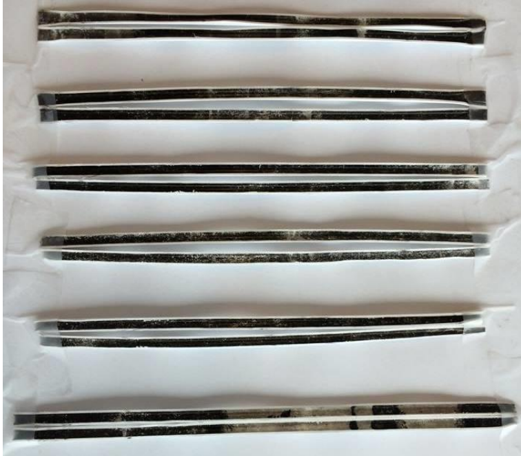
Figure 4-6: Autopsy photo of a representative membrane fiber cut in 6 pieces after 46 filtration and backwash cycles.
