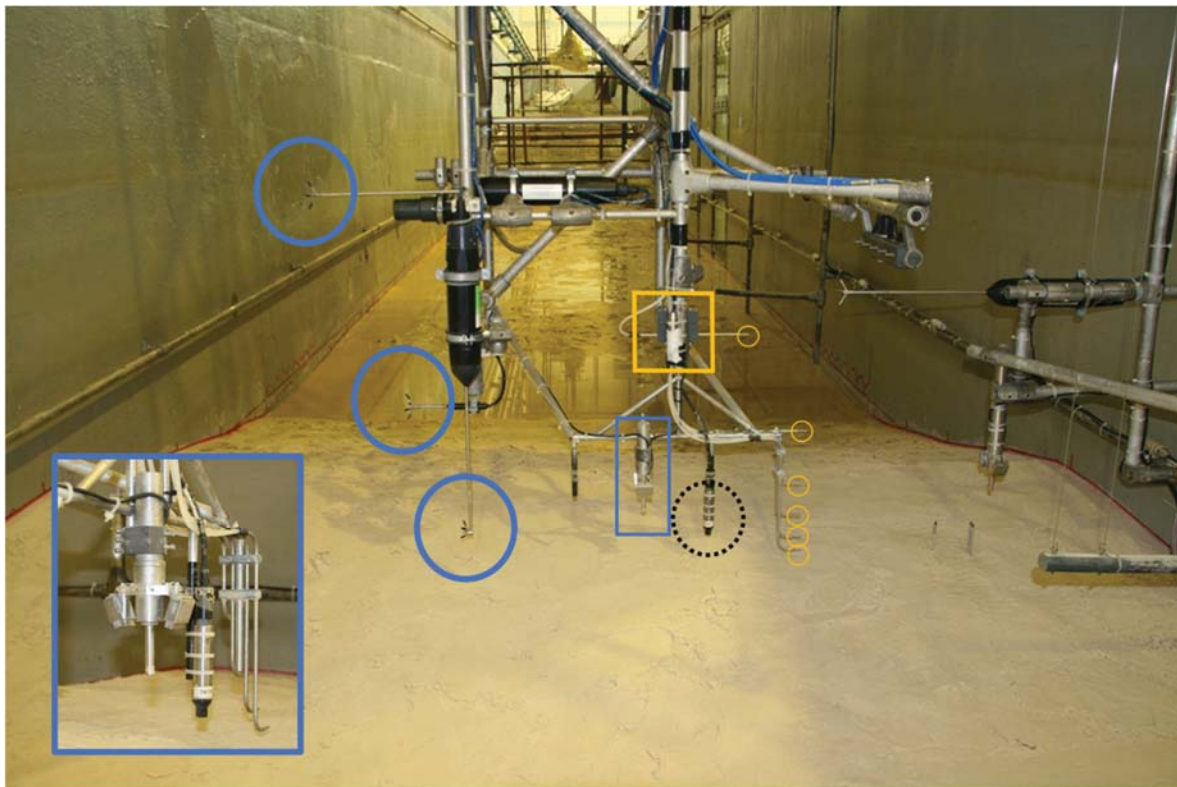
Figure 3.2. Mobile measuring frame and instrumentation. Instrumentation includes three ADVs (blue solid circles), one Pressure Transducer (yellow square), a six-nozzle Transverse Suction System (yellow circles), an OBS (black dashed circle) and an ACVP (blue square). Inset shows close-up of near-bed instrumentation.
