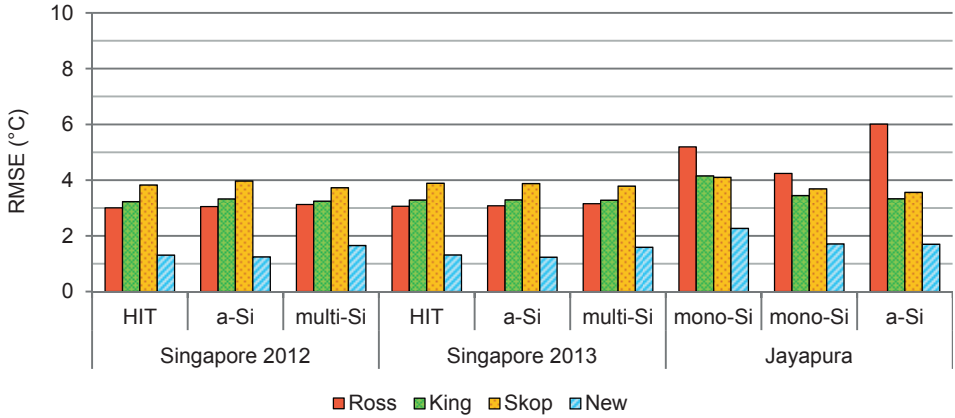
Fig. 7.13. RMSE of the measured vs. simulated PV module temperature (°C) for various PV modules and models.
