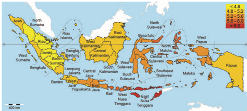
Fig. 2.9. Average daily irradiation in kWh/m 2 for each province in Indonesia. Names of provinces are shown in map. These data were obtained from the NASA Langley Research Center Atmospheric Science Data Center Surface meteorological and Solar Energy (SSE) web portal supported by the NASA LaRC POWER Project.
