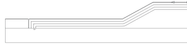
(b) Tool paths generated for the product adjacent boundary by standard profiling
