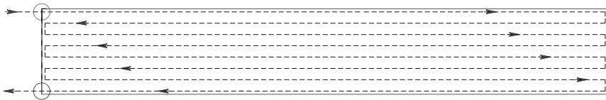
Figure 4.21: Another example tool path for a moderately long machining feature.
