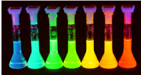
Figure 2.5: Cadmium selenide quantum dots fluorescence at different wavelengths, taken from Ref. [24].
