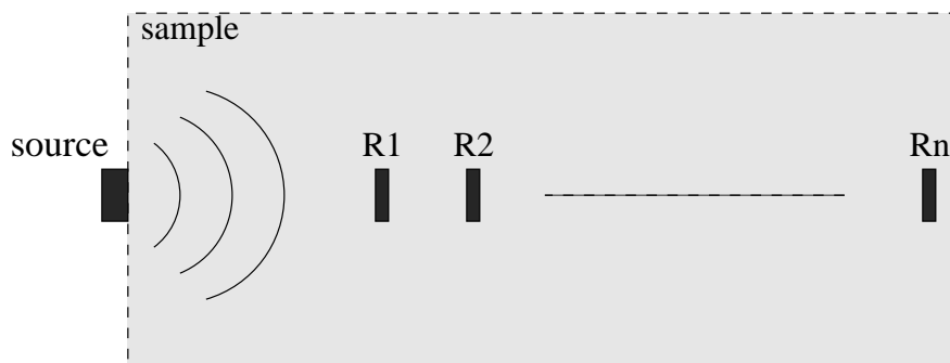
Figure 2.1: Sketch of a source and receivers ( R_1, R_2, \dots, R_n ) in a configuration allowing for the application of the spectral ratio technique .
