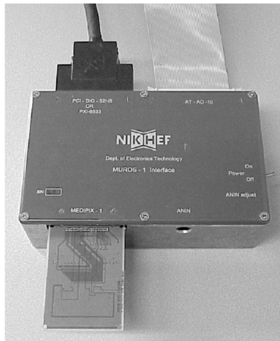
Figure 3.7: The Muros1 board interfaces a Medipix1 chip to a PC.
