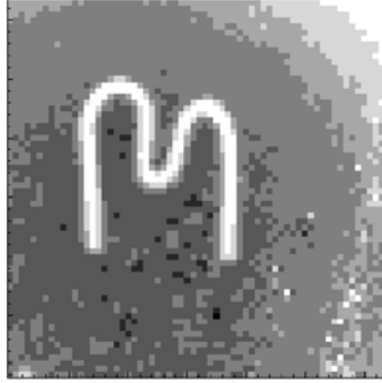
Figure 3.14: One of the first Medipix1 raw images using a ^{90}\text{Sr} source (electrons). The different colours represent different numbers of counts per pixel. The image is formed by a 500\ \mu\text{m} thick tungsten wire bent to an m character. A chip bonded to a 200\ \mu\text{m} thick GaAs sensor was used. This image has subsequently been adopted as official logo by the Medipix collaboration [24].
