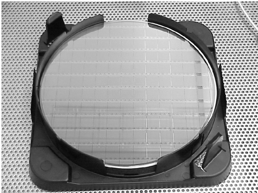
Figure 5.15: A 200 mm diameter wafer contains 94 Medipix2 chips.
