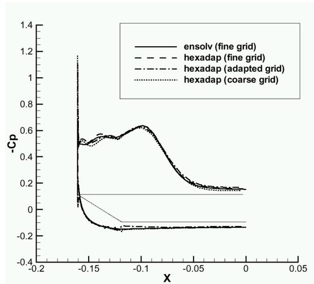
Figure 3: Vortex flow over a delta wing ( $Re=40,000$ ,  $M=0.3$ ,  $\alpha = 12.5^\circ$ ). Comparison of pressure coefficient at a cross section of 60% chord between the DG solver Hexadap and the finite volume solver ENFLOW. For Hexadap results are also shown on the unadapted coarse and fine meshes.
