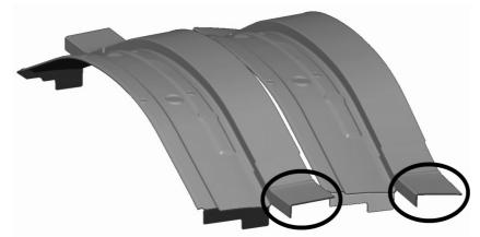
Figure 3.: Tool geometries: left original, right compensated, note the smoothly compensated flanges.
