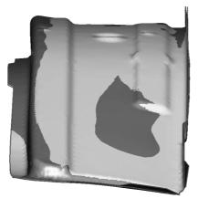
**Figure 2.:** Part geometry after springback (light grey) and after application of the smooth displacement field (dark grey) (exaggeration factor 5)
