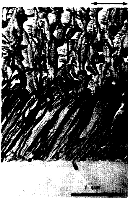
Fig. 25. Replica electron micrograph of an obliquely-evaporated Fe film ( \alpha_i=65^\circ , T_s=473 K, evaporation rate= 0.83 nm s^{-1} , background pressure= 0.13 Pa). (Taken with permission from ref. 54).
