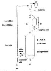
Fig. 4. Schematic representation of the small scale CFB unit.
