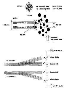
Fig. 2. Schematic representation of the optical probe system, containing two multi-fibre sensors.
