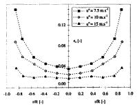
Fig. 10. Local solids concentration as a function of dimensionless radial position at 1.8 m above the solids distributor for three superficial gas velocities;  $G_s = 300 \text{ kg m}^{-2} \text{ s}^{-1}$ .
