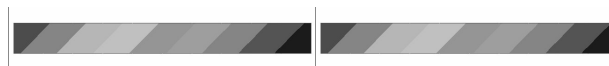
Fig. 3. The initial linear field of the equivalent plastic strain (left) and the final field (right).
