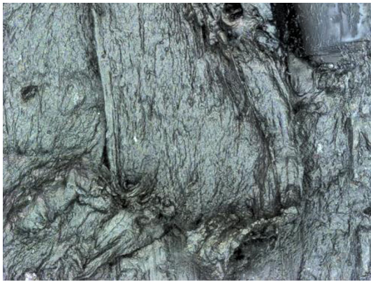
Fig. 14 Confocal microscopic picture of a polluted rough granite sphere in contact with MS
