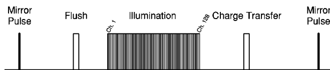
FIG. 6. Timing diagram of an experiment recording a full sequence of 128 images. The CCDs are illuminated by the mirror for about 31% of the time between successive mirror pulses. The repetition time of the mirror pulses has a range of 17\text{--}500 \mu\text{s} . In this mode of operation, all CCDs are flushed before the illumination and charge transferred after the illumination. Readout is performed after charge transfer.
