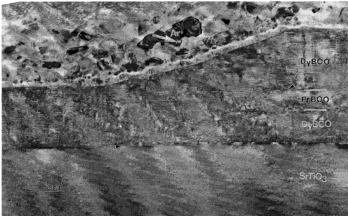
Fig. 2. A TEM image of a ramp-edge junction DyBCO/PrBCO/PrBCO/DyBCO on a \text{SrTiO}_3 substrate facing towards the JJ ion gun. The interfaces between the layers are indicated by solid white lines. The horizontal lines correspond to (001) fringes with a spacing 1.17 nm. The barrier layer is indicated by two black arrow heads. All components of the device are c oriented and epitaxial to the [001] direction of the substrate. A substrate ramp can be observed.
