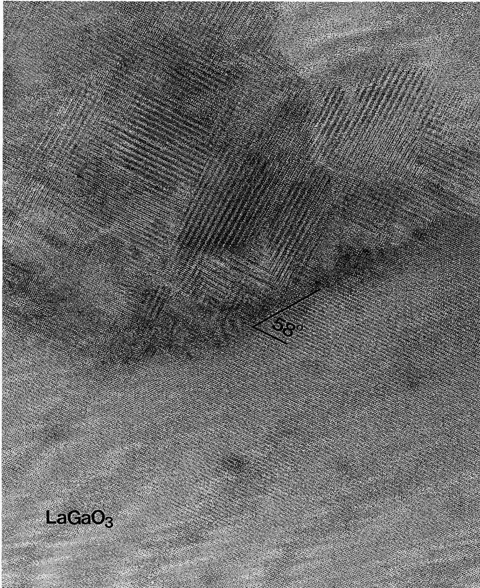
Fig. 11. An YBCO thin film grows on a step with step angle around 45^\circ with a mix of a and c oriented grains.
