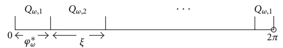
FIGURE 4: An illustration of a b -bit APQ in the phase domain, where Q_{\omega,j} , j = 1, \dots, 2^b denotes the j th quantization interval with width \xi , and offset angle \varphi_{\omega}^* . The first interval Q_{\omega,1} is wrapped.
