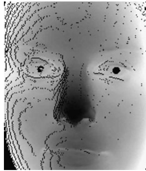
Fig. 15 High resolution range image. For the black areas , no depth information is available in the original point cloud
