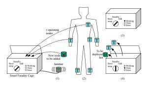
**Figure 3.** Procedure for adding a node where  $\tau = 2$
