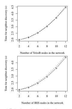
Figure 6. Timing figures for the neighbor discovery protocol (Protocol 2) on TelosB and IRIS. Dashed lines represent prediction using (2).
