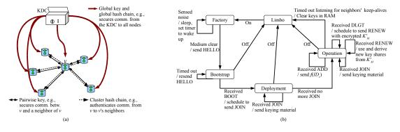
Figure 1. (a) Essential key types; (b) simplified finite state machine of a node connecting the different phases
