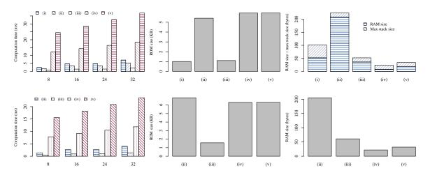
Figure 4. Performance and resource usage of (i) hardware AES-CBC-MAC, (ii) software AES-CBC-MAC, (iii) Skipjack-CBC-MAC, (iv) TuLP, (v) TuLP-128 on TelosB (top row) and IRIS (bottom row). Note: IRIS does not support hardware AES-CBC-MAC; stack size information is not available for IRIS.
