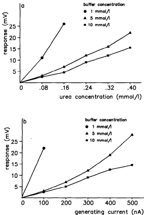
Fig. 9. A comparison between (a) enzymatically and (b) coulometrically induced pH changes in dependence of the buffer capacity of the solution.
