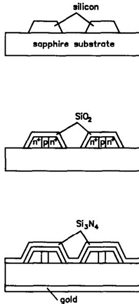
Fig. 3. Diagram to show that in the Silicon on Sapphire technology (SOS), transistors are fabricated in small silicon islets, deposited on an insulating Al<sub>2</sub>O<sub>3</sub> substrate.
