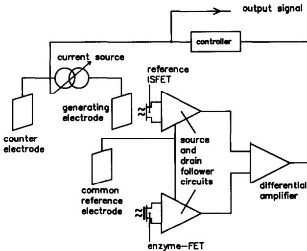
Fig. 10. Coulometric control system in which the pH at the reference-ISFET is kept equal to that at the ENFET.
