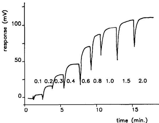
Fig. 7. Time response of urease/albumin ENFETs. The sensor output is sensitive to the stirring of the solution after each addition of urea. The figures at the curve indicate the urea concentration in  $\text{mmol litre}^{-1}$ .
