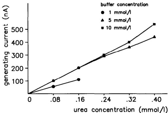
Fig. 11. Generating current as a function of urea concentration for the system depicted in Fig. 10. Only for small pH changes the system is insensitive to the buffer capacity.
