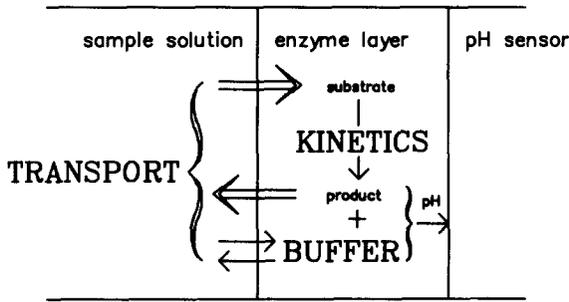
Fig. 2. Diagram to illustrate that the response of pH-based enzyme sensors is governed by the transport rates of the chemical species, the enzyme kinetics and the buffer capacity of the sample.
