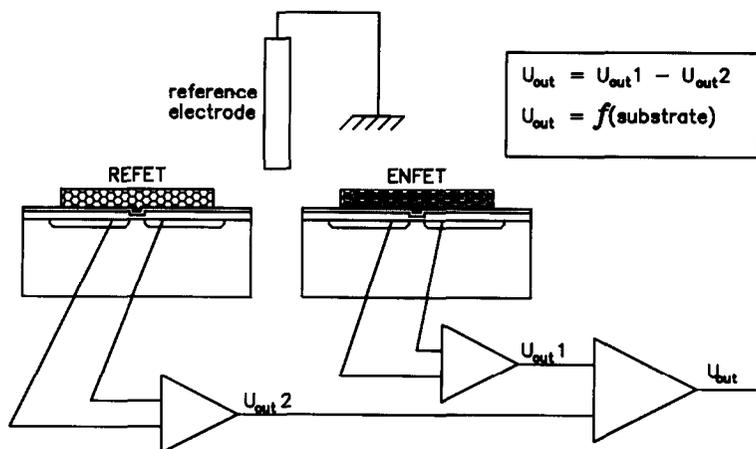
Fig. 1. Experimental set-up for ENFETs using one ISFET with an enzyme loaded membrane as the sensor and one ISFET with an unloaded membrane as a reference.
