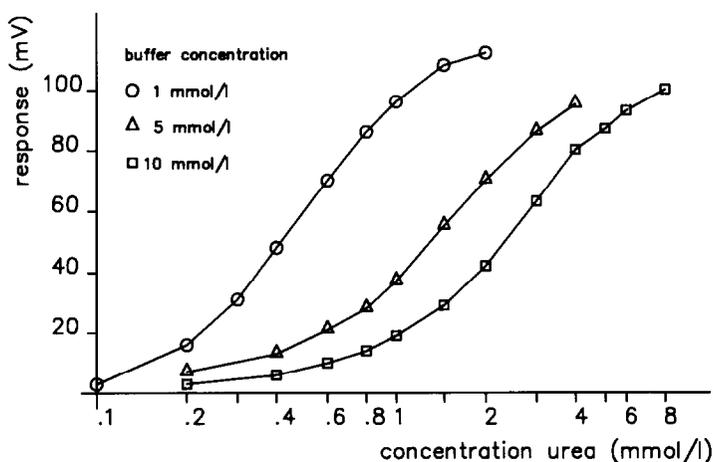
Fig. 8. Graph showing that the sensitivity and dynamic range of the urea-ENFET depend on the buffer capacity of the sample.
