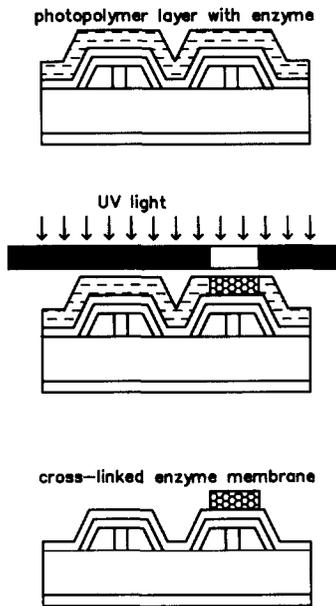
Fig. 4. Diagram to show the use of photo-sensitive PVA for the selective deposition of enzyme membranes over the ISFET gate areas.
