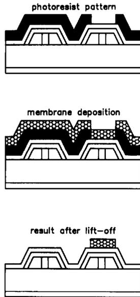
**Fig. 6.** Diagram to show that the lift-off technique can be used to pattern membrane materials that are not photo-sensitive themselves.
