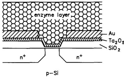
**Fig. 12.** Schematic cross section of the pH-static enzyme sensor. The enzyme membrane is deposited over the entire structure.
