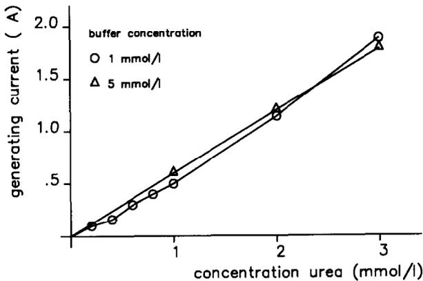
**Fig. 13.** Graph showing that the output of the pH-static enzyme sensor is independent of the sample buffer capacity and the dynamic range is expanded.
