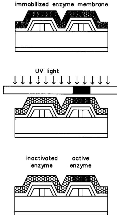
**Fig. 5.** Diagram to show that through the local inactivation of immobilized enzymes, ENFETs and reference-FETs are fabricated on the same chip without the need for patterning the membrane.
