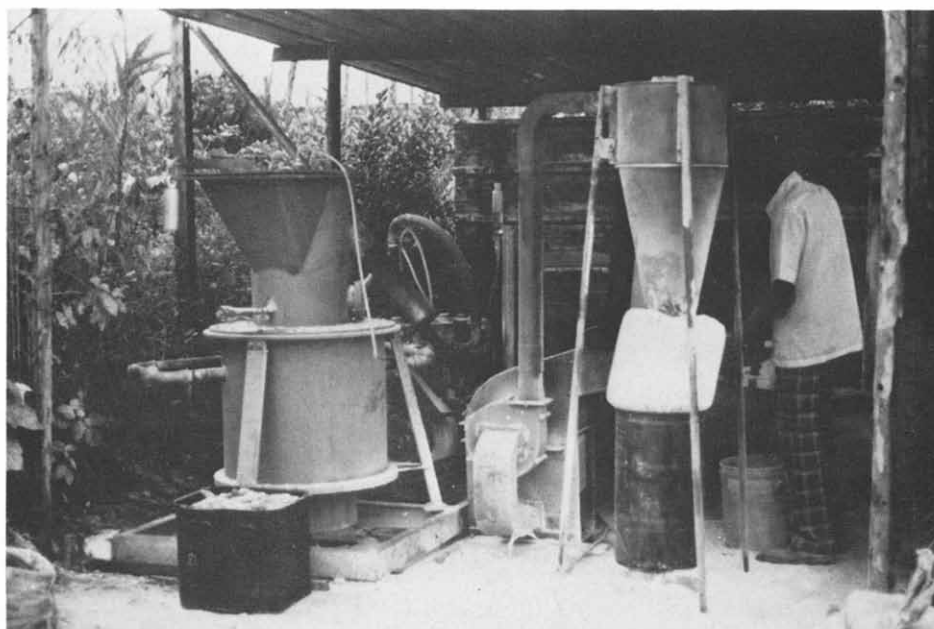
Fig. 9. Application of biomass gasification in Tanzania. Maizepills are gasified to generate energy for maize milling.
