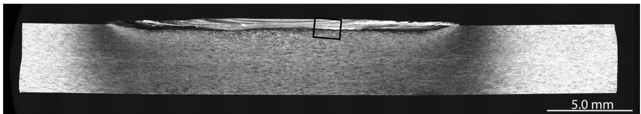
Figure 4. Macrostructure of the transverse cross section after the cladding experiment.
